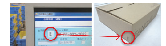
A computer screen displaying the optimum delivery box size at the delivery area
