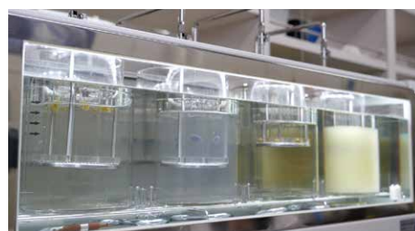
Disintegration test machines used for pharmaceuticals are also able to reproduce the way in which supplements dissolve in the stomach
